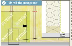
Unroll INTELLO for entire wall section allowing sufficient material for "relaxed" corners, returns onto intersecting wall studs and fixing to joinery. Preferably cut wall sections after stapling main sections of INTELLO. Important: The writing on the INTELLO should face into the room
