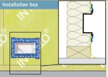
Cut a hole in the INTELLO that is the same size as the INSTAABOX. Make the required number of holes in the INSTAABOX and feed the cable through these holes, then align the INSTAABOX and tape it to the INTELLO with TESCON VANA, ensuring that you form an airtight seal.
